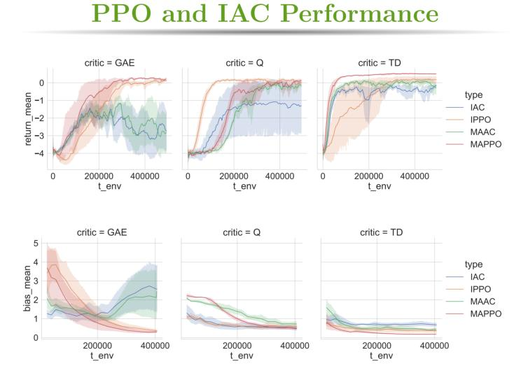
The plot shows that, for all critics, the bias is lower for the PPO version of the critic than the actor-critic version. A possible explanation for this is that clipping the actor makes the returns distribution more predictable and therefore easier to learn.
